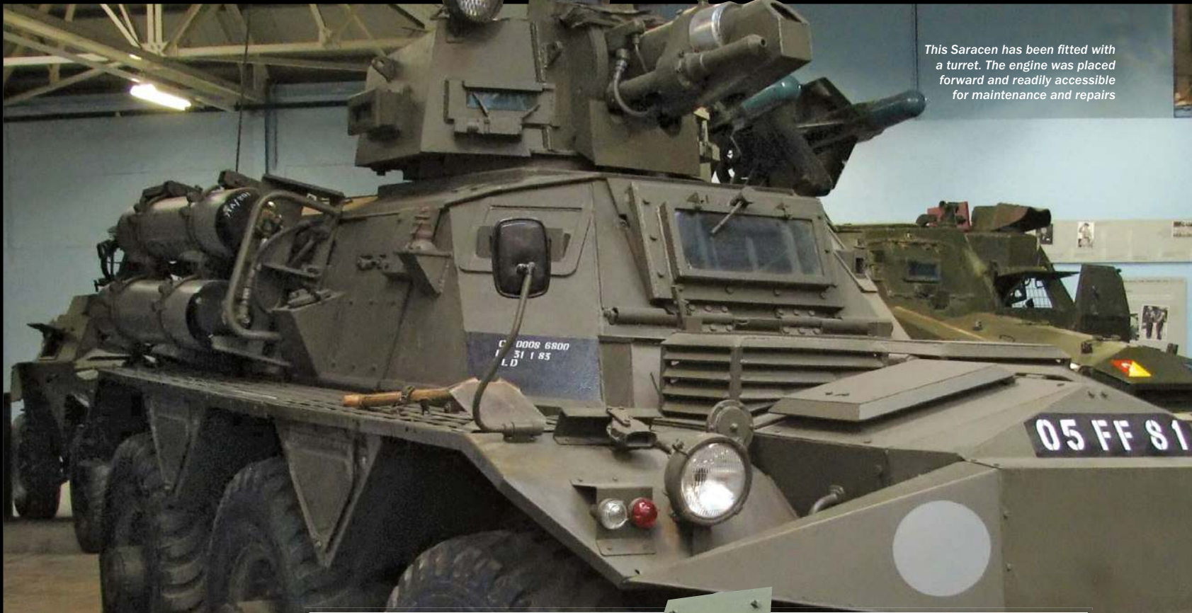
The small turret crowning this Saracen was capable of mounting a water cannon or machine gun. Also note the firing ports that allowed troops to engage the enemy from within
